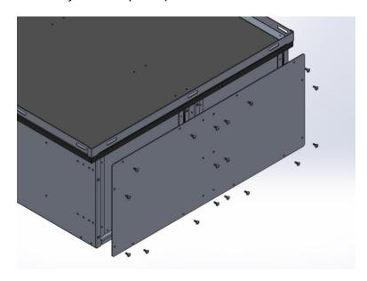
**STEP 2** Place drawer unit on previously installed base, and align mounting holes in the cabinet with ¼" threaded inserts in the base, number of mounting points depends on unit size. (Extend drawers if back panel removed for access to mounting holes)
