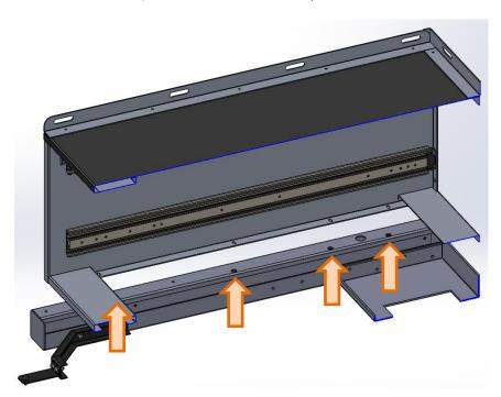
**STEP 3** Mount the drawer unit to the base using the provided ¼" hardware; 1x bolt, 1x washer.
