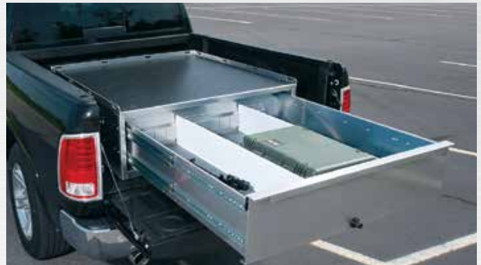
Full drawer extension with push button lockout
