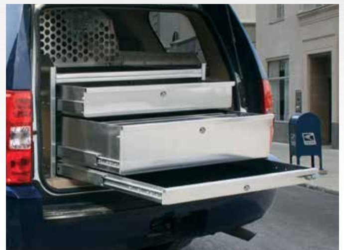
Custom stacked three drawer command unit with optional partition. Third drawer is map/command board. Model#: OPC-CTU-24-47-36-DY3
