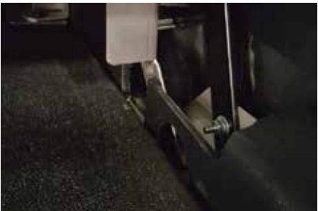
Elevated mounting brackets allow quick access to spare tire.
