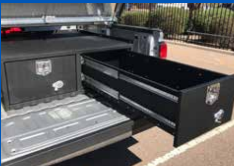
The Dual Drawer Series with Simplex lock. Model: OP-TDU-15-48-48-101
