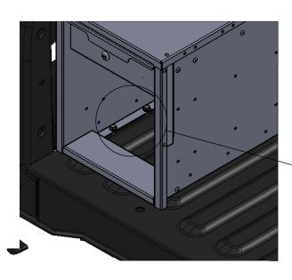
STEP 3: DRILL THROUGH BOTTOM FLANGE IN CABINET SIDE PANELS AND USE 5/16" BOLTS, WASHERS, AND NYLOC NUTS TO FASTEN TO TRUCK BED
