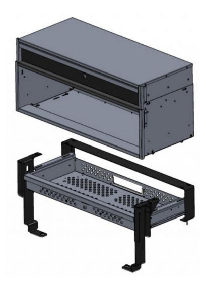
1. AFTER THE BRACKETS ARE INSTALLED IN THE VEHICLE, THE RADIO TRAY AND THE PDU UNIT ARE FIXED TO THE BRACKETS TOGETHER.
