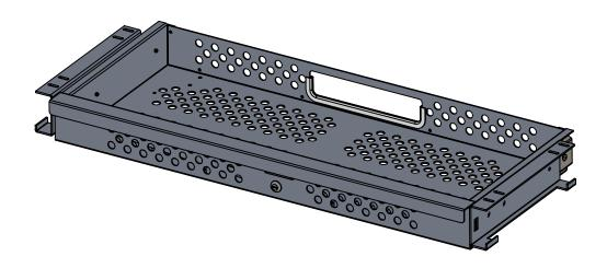
STEP 1: REMOVE THE BOTTOM DRAWER OF PDU UNIT BY OPENING IT TO FULL EXTENSION AND PUSHING THE PLASTIC TABS IN OPPOSITE DIRECTIONS LOCATED ON BOTH SIDES OF THE SLIDE WHILE PULLING THE DRAWER STRAIGHT OUT.
