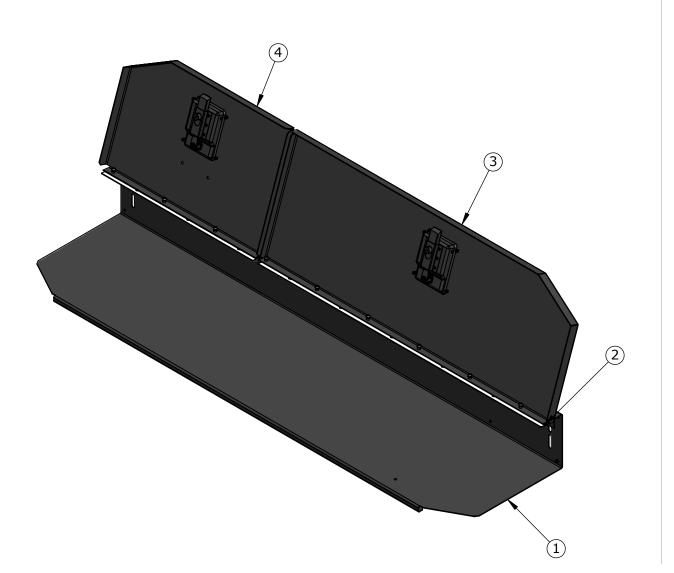
ASSEMBLY STEP-2: THEN PUT THE FRONT PANEL, STIFFNER AND PARTITION.
