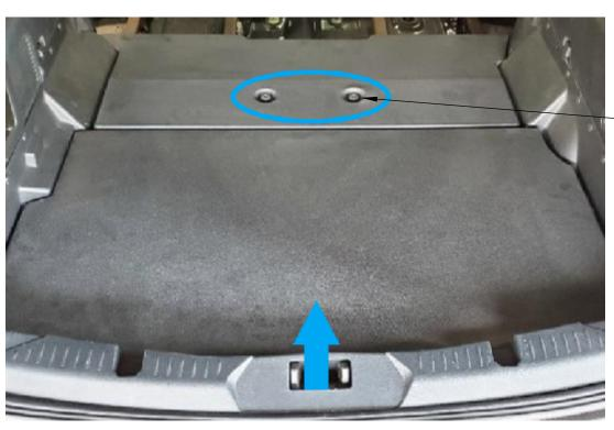
STEP 1: REMOVE THE FRONT SECTION OF OEM TRUNK FLOOR
