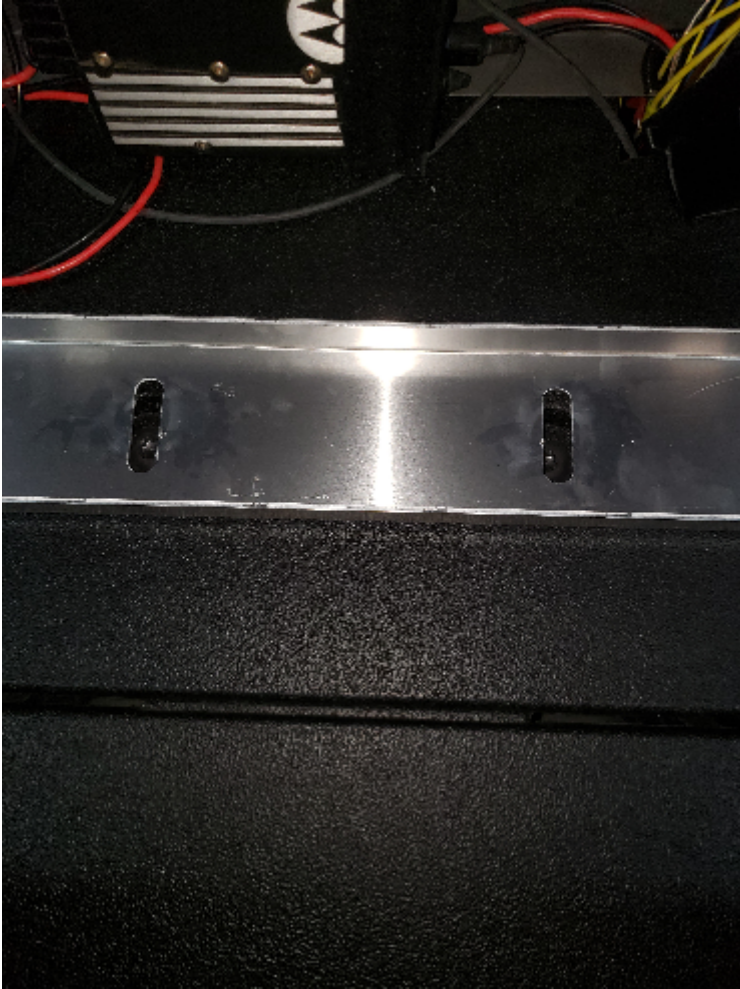
ALIGNMENT OF REAR LOOP BRACKET AFTER PLACING BACK THE TRUNK FLOOR
