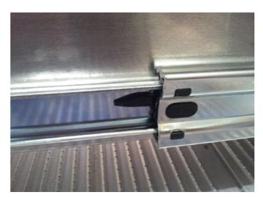
STEP 2: REMOVE BOTTOM DRAWER USING TABS ON SLIDES
