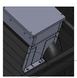
STEP 4: DRILL THROUGH BOTTOM FLANGE IN REAR SUPPORT AND USE 5/16" BOLTS, WASHERS, AND NYLOC NUTS TO FASTEN TO TRUCK BED
