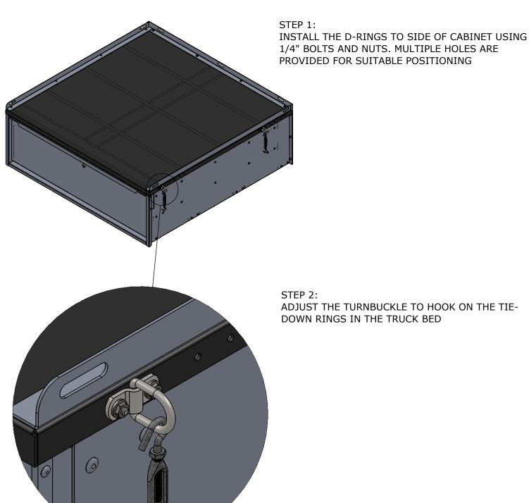
STEP 2: ADJUST THE TURNBUCKLE TO HOOK ON THE TIE-
